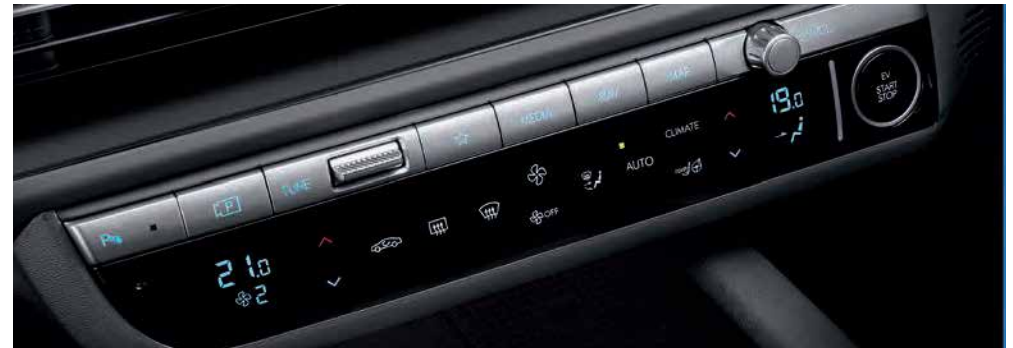
Dual-zone Full Automatic Air Conditioning
